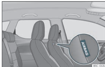
Fig. 19 In the inner padding of the driver's seat backrest: central airbag.
