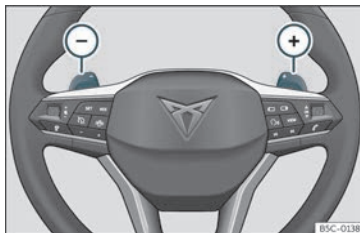
Fig. 138 Steering wheel: automatic transmission levers
