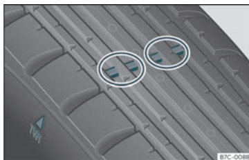
Fig. 194 Tyre profile: tread wear indicators.
