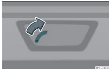
Fig. 81 Detail of the luggage compartment: emergency unlocking
