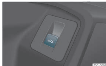
Fig. 79 On the driver's door: button to open and close the rear lid.
