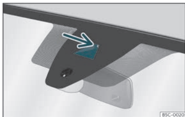
Fig. 142 On the windscreen: field of vision of the Lane Assist system.
