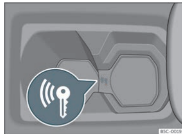
Fig. 135 In the centre console: emergency start. »
