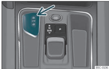
Fig. 66 Centre console: vehicle key socket.
