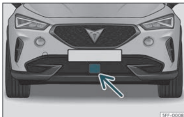
Fig. 140 On the front bumper: radar sensors.
