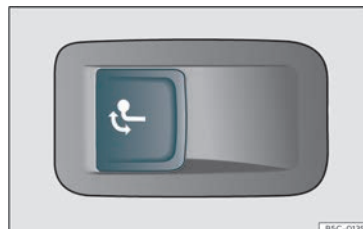
Fig. 179 On the left side of the luggage compartment: button for unlocking the tow hook.
