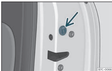
Fig. 75 Locking the door manually.
