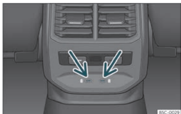
Fig. 133 Rear part of the centre console: USB connectors with power outlet function.
