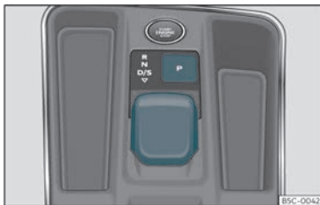
Fig. 137 In the centre console: selector lever.
