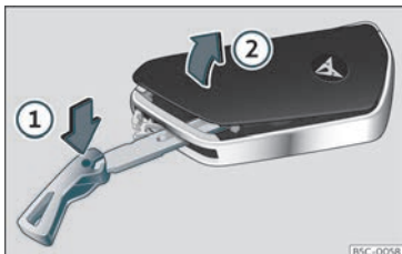
Fig. 68 Vehicle key: opening the battery compartment cover.
