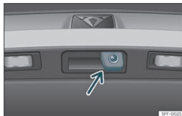
Fig 145 In the rear lid handle: location of the reverse assist camera.
