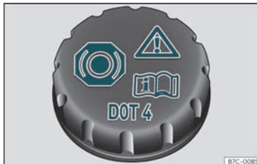
Fig. 190 Engine compartment: brake fluid reservoir cap.
