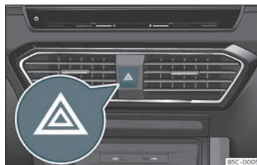
Fig. 87 Dash panel: hazard warning lights switch
