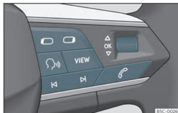
Fig. 56 Right side of the multifunction steering wheel: buttons for using the instrument cluster's menus and information displays (depending on versions).
