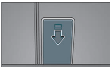
Fig. 116 In the luggage compartment: opening the trapdoor.
