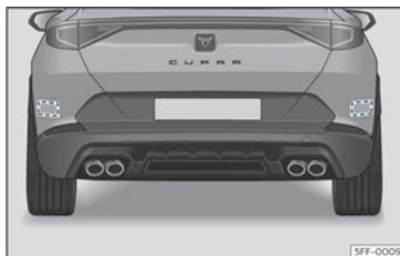
Fig. 143 Rear view of the vehicle: radar sensor zones.
