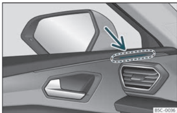
Fig. 160 Control lamp of the lane departure warning.
