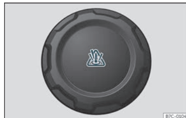
Fig. 189 Engine compartment: coolant expansion tank cap.
